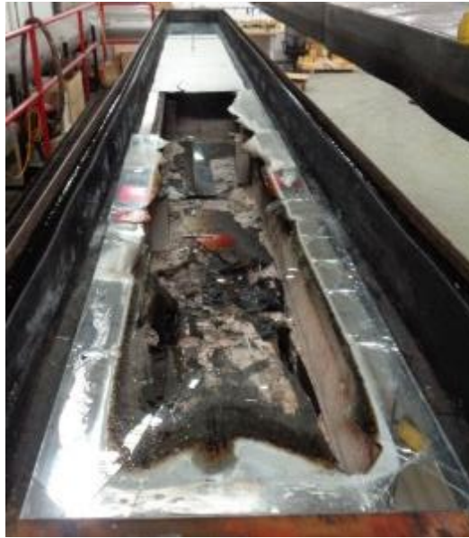
Photo No. 3 Unexposed Surface of the Test Specimen (Post-test)
