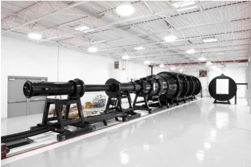
Figure #1 Shock Tube and Test Facility
