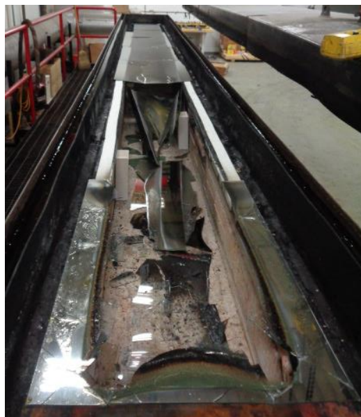
Photo No. 4 Exposed Surface of the Test Specimen (Post-test)
